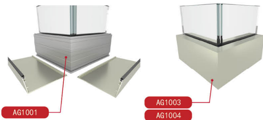
转角位置安装 Splicing Installation Method
